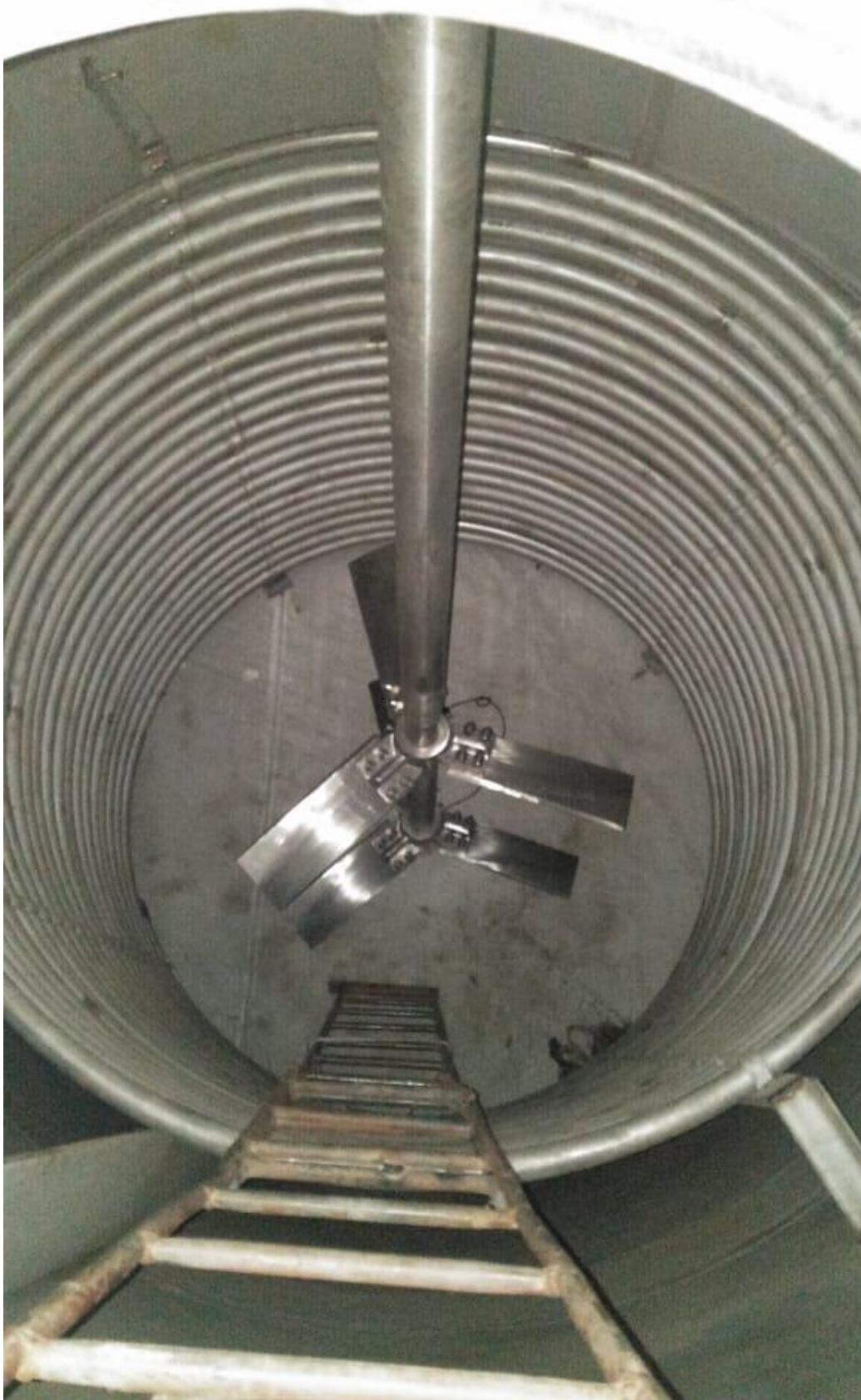
Agitator Assembly In Reactor
