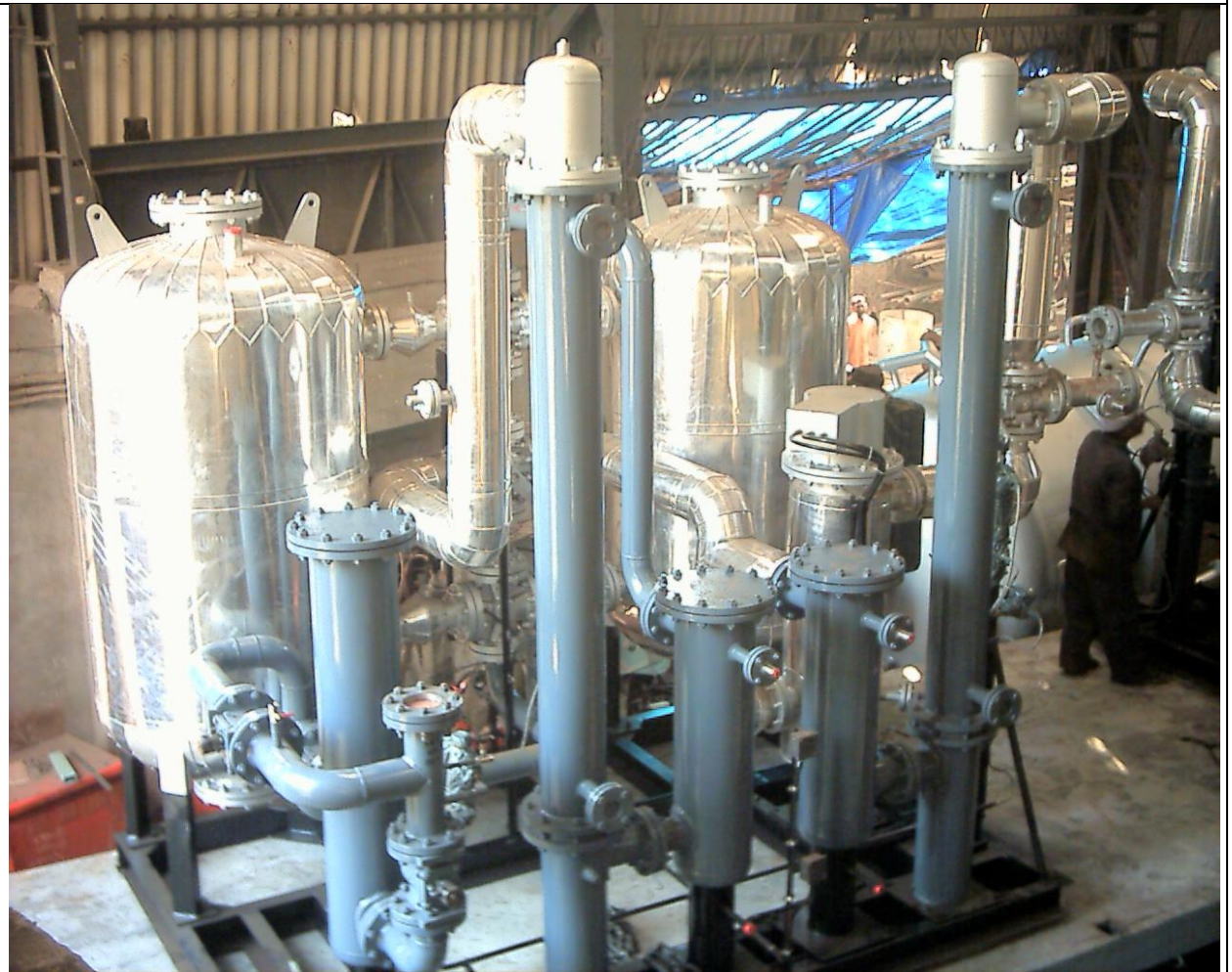
Air Dryer In Skid Mounted Assembly
